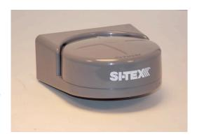
The CDK-11 also provides compatible electronics with pitch and roll data for accurate, stable heading performance. Static pitch and roll accuracy is <1°, with dynamic pitch and roll accuracy rated at <3°. The CDK-11 outputs heading data at 10Hz in NMEA0183, adjustable up to 20Hz. The CDK-11 can also output heading data in NMEA2000<sup>®</sup>.
